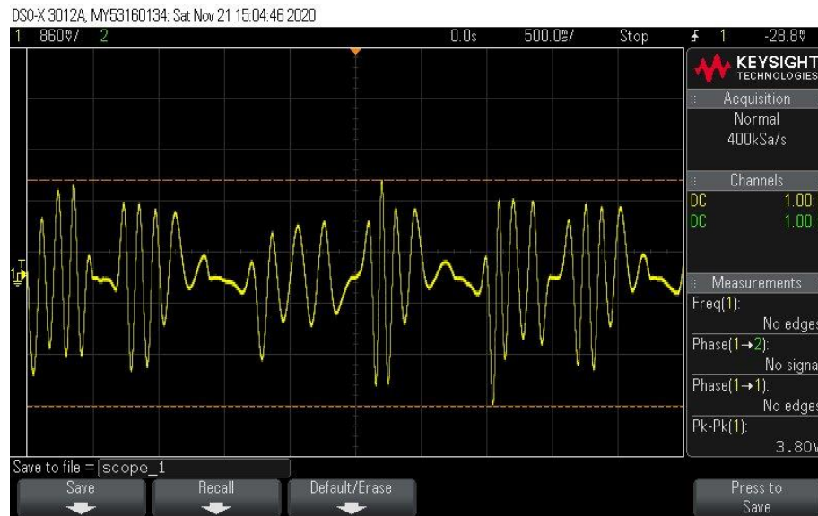
Figure 16. Oscilloscope capture of point absorber generator at steady motion
